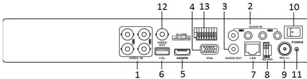
\*: The rear panel of DS-7208/7216HUHI-K2/P provides 8/16 video input interfaces.
